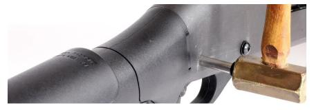
Slip a washer over one of the buttonhead screws and thread it into the ejection port side of the standoff.
