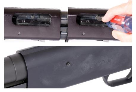
Put the factory ejector screw in a safe place with the factory trigger pin.
