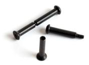
It is important to realize that once the Chicago screws are tightened against each other, they are not going to get any tighter, and applying too much torque will snap them at the center. It is useful to practice tightening them outside the shotgun before installation, to get a feel for how tight they can get, and also to clean the threads of any dirt or debris.
