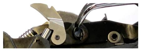
Reinstall the trigger group and put the buttonhead Chicago screw and washer through from the ejection port side.
