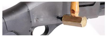
Sometimes the Chicago screw will not slide through the trigger group. It hangs on the pin retainer wire that is visible if you look through the hole. If this happens, remove the trigger group (you will have to remove the rear trigger pin) to get access to the pin retainer wire. Remove the pin retainer with a needle nose pliers or even a flathead screwdriver.
