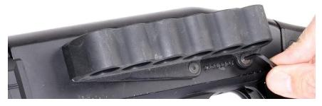
If the Chicago screws are tight, but the shell carrier is not, consult the section on Chicago screws at the front of this manual.
