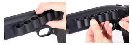
While holding the shotgun so the shell carrier assembly is facing up, slip the female Chicago nut through the SureShell bracket and into the trigger pin hole. The screws have been sized so that they can be firmly tightened with the hex keys without fear of squeezing the action. You can make the screw finger tight with the long arm of the hex key. A drop of purple of blue thread lock on each screw will keep it in place. Be sure to check for loose screws every time you use your shotgun.
