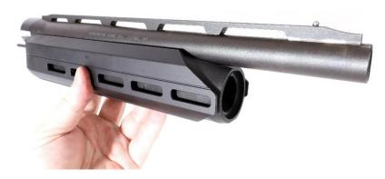
17. Install the barrel assembly with forend onto the shotgun While holding the front cap in place, slide the barrel assembly with the forend over the magazine tube. Again, though a little awkward, it is best to do this with the muzzle facing down, in case the front cap separates from the forend. But if you hold the front cap securely it should stay in place.
