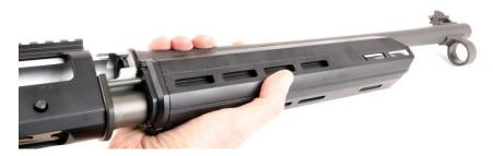
You should be able to re-install the barrel, fitting the rear boss of the rear end cap into the forend support plate on the front of the shotgun receiver. If your shotgun is fitted with the factory magazine extension and spacer, ensure it is aligned with the magazine and forward barrel ring as you slide the barrel and forend assembly into place, then screw it finger-tight onto the magazine. Tighten the complete barrel and forend assembly down with the magazine cap.
