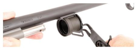
The factory front sling loop is retained by a c-clip or snap ring that can be removed with snap ring pliers. Once the c-clip is removed you can slide the front sling loop off over the front of the barrel.
