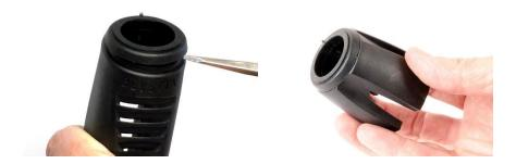
The detent ring assembly is installed on the nose of the factory forend. Carefully remove this from the forend with a flat blade screwdriver. The o-ring surrounding the mounting tabs is not required for the Truckee forend installation and can be removed.
