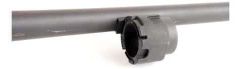
6. Slide the aluminum forend along the barrel to seat in the rear of the front end cap
