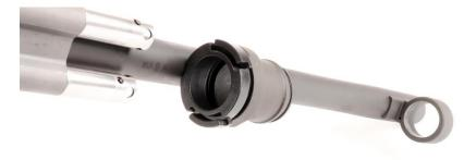
If your shotgun is fitted with the factory magazine extension and spacer, slip it into the forward barrel ring now and let it hang loosely.
