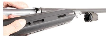
Carefully slide the aluminum forend past the rear barrel flange, gas cylinders and rear barrel ring until the inner flange of the forend seats itself in the upward-facing slots in the front end cap you just installed.
