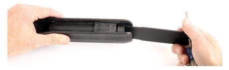
If the forend nut is very tight, it is quite possible you will twist the action bars (or even the forend wrench) slightly while trying to remove the forend. The action bars can be easily restored to straightness by hand
