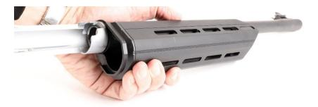
9. Reinstall the barrel and Truckee forend on the shotgun Slide the barrel and forend assembly back onto the shotgun, forcing the rear end cap past the bulging ring on the magazine. When reinstalling the magazine extension, orient the factory sling loop so it is facing down and does not interfere with the Truckee forend.
