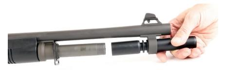
3. Remove the factory front sling loop (optional)
