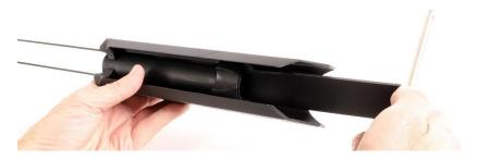
Once it is started, use the forend wrench to tighten the nut about a quarter turn past the point when the front end cap is fully engaged. The nut should be pretty tight on the assembly and of course there should be no movement.
