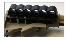
Now line up the two rear standoffs with the rear horizontal sling loop, and secure the assembly in place with two  $\#10-32\times7/16$  inch button head cap screws passing through the sling loop and the two #10 washers. Tighten the assembly with both hex keys at the same time.
