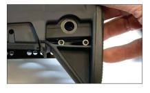
Now line up the two rear standoffs with the sling loop, as far reward as possible, and press the standoffs into the slot. Use the 9/64 inch hex key to thread the #8-32×7/16 inch socket head cap screws through the sling loop and into the standoffs. Tighten the assembly with both hex keys at the same time.
