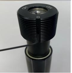
**3. RB5100 Adjustment Instructions:** There are three different setting options on the buffer, 0 (open), MD (Medium Damped), and HD (Heavy Damped). To select the damping, loosen the set screw on the side of the cylinder with the .050 hex key provided with the buffer.
