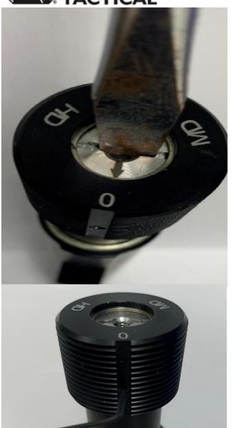
4. Once set screw is loosened, use a flathead screwdriver to select the damping level by twisting the adjustment knob. (located at the top of the buffer)
