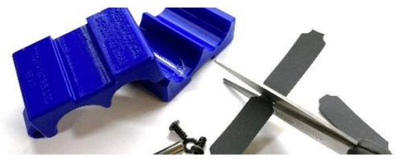
Then adhere the gasket strips to the inside of the vise blocks:
