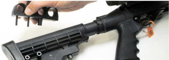
3. Put the longer screws through the rear mounting holes, the unthreaded hex standoffs and the buttstock's sling slot to screw them into the steel mounting cleat. Push the assembly as far forward as possible be-
