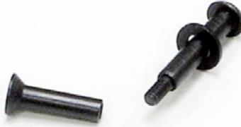
It is important to realize that once the Chicago screws are tightened against each other, they aren't going to get any tighter, and applying too much torque will snap them at the center. It is useful to practice tightening them outside the shotgun before installation, to get a hang for how tight they can get, and also to clean the threads of any dirt or debris.
