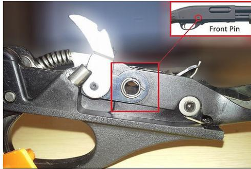
5. The front clip on the 870 trigger assembly is designed to hold the factory trigger pin in place. Our Chicago screw DOES NOT require a clip. To install the front Chicago screw on the Remington 870 you will need to remove this clip and keep it with your factory trigger pins.
