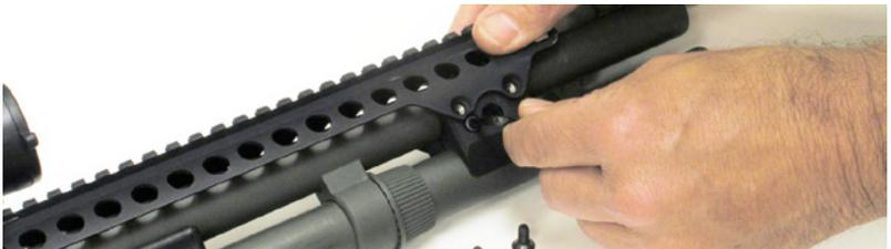
The fit between the rail and the clamp is very tight. The best installation procedure is to *loosely* install the clamp in its approximate location before attaching the rail at the receiver. Once the rail is firmly mounted on the receiver (or on the stock adapter for High-tube full length rails), move the clamp until the rail mounting holes are lined up and the mounting screws are started before finally tightening it into place. Use blue Loctite on all fasteners.
