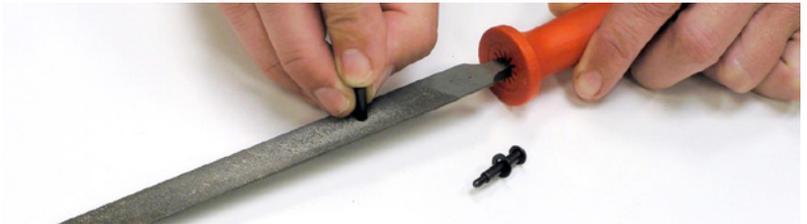
Chicago screws can benefit from a drop of blue Loctite® on the threads.
