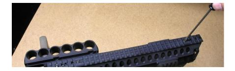
Now fully tighten the M4 button head screws and the angled set screws.
