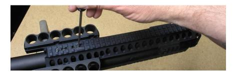
Once you have established that everything fits well together, we suggest you disassemble the SureShell Carrier and Rail for the KelTec KSG and re-assemble it once again, putting a drop of blue or purple thread locker on each threaded fastener.
